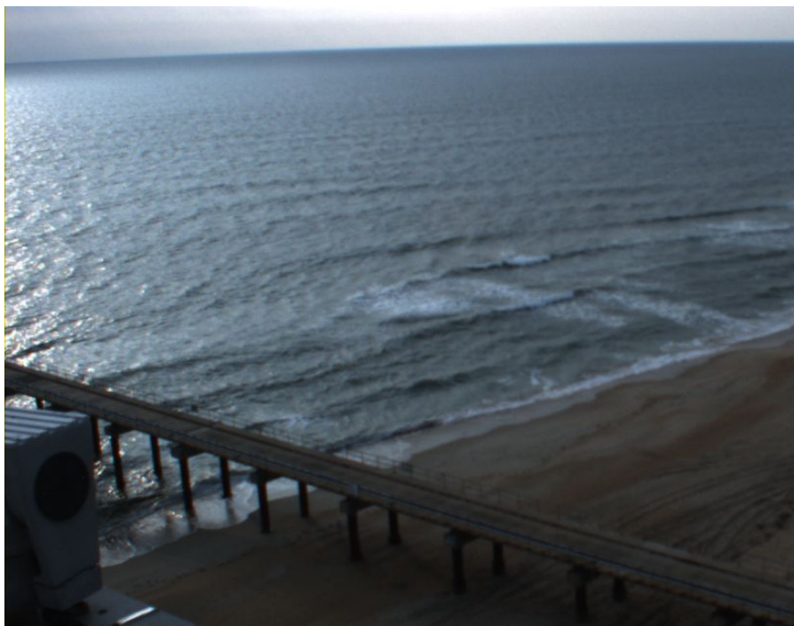
Fig. 1 Snapshot from Duck, NC, USA showing the wide range of scales of optical variability. Because optics depend on sea surface slope, high frequency chop dominates measured signals and must be mitigated by appropriate signal processing.
