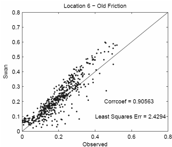
Fig. 1a Scatter plot showing correlation between the default SWAN friction routine and the observed data at Lake George
