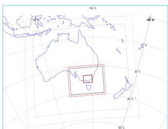
**Figure 1:** Spatial dimensions of the three domains, the outer domain at 50 km resolution, the intermediate domain at 10 km resolution and the innermost convective permitting resolution domain (at 2 km resolution). The red markers denote the native model domain and the black markers indicate the model domain after the relaxation zone of 10 grid cells is removed
