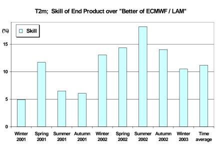
Mean Absolute Errors of End Product and DMO temperature forecasts (left), and Skill of the End Products over model output (right). The better of either ECMWF or local LAM is chosen up to the +48 hour forecast range (hindcast), thereafter ECMWF is used. The figure is an example of both aggregation (3 stations, several forecast ranges, two models, time-average) and stratification (seasons).
