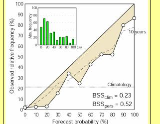
BS =  $(1/n) \Sigma (p_i - o_i)^2$ BSS =  $[1 - BS / BS_{ref}] * 100$ RPS =  $(1/(k-1)) \Sigma \{(\Sigma p_i) - (\Sigma o_i)\}^2$ RPSS =  $[1 - RPS / RPS_{ref}] * 100$ ROC\_SS =  $2 * ROC_A - 1$
