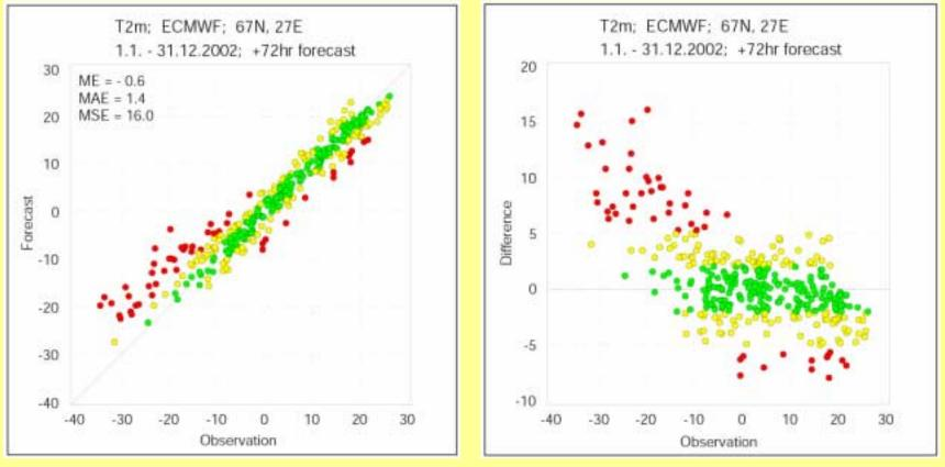
Scatterplot of one year of ECMWF three-day T2m forecasts (left) and forecast errors (right) versus observations at a single location. Red, yellow and green dots separate the errors in three categories. Some basic statistics like ME, MAE and MSE are also shown. The plots reveal the dependence of model behaviour with respect to temperature range, i.e. over- (under-) forecasting in the cold (warm) tails of the distribution.
