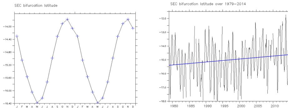
Figure 4: Seasonal climatology SEC bifurcation latitude calculated from 3-month running mean of monthly model output (left). Time series of SEC bifurcation latitude and its linear trend (right).
