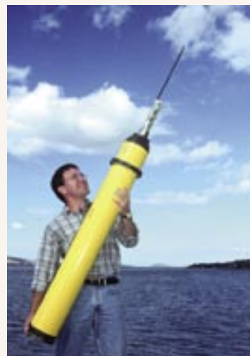
Figure 6: An Argo float (CSIRO).
