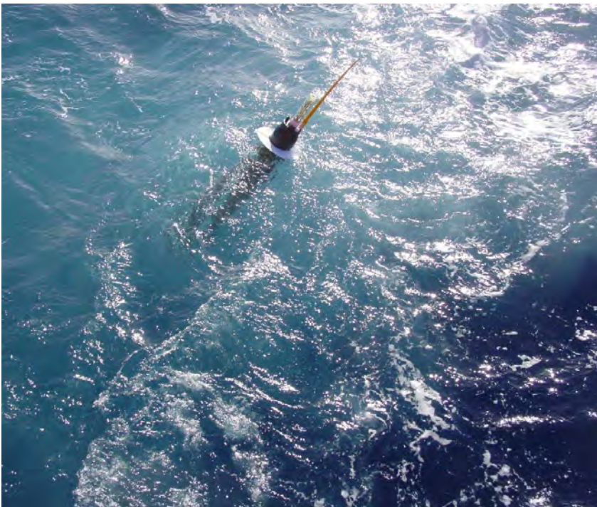
Figure 3. Argo floats are battery-powered autonomous devices that drift in the sea collecting high-quality temperature and salinity profiles from the upper 2000 metres of the ice-free global ocean. The ocean data are transmitted via satellite to scientists on shore.
