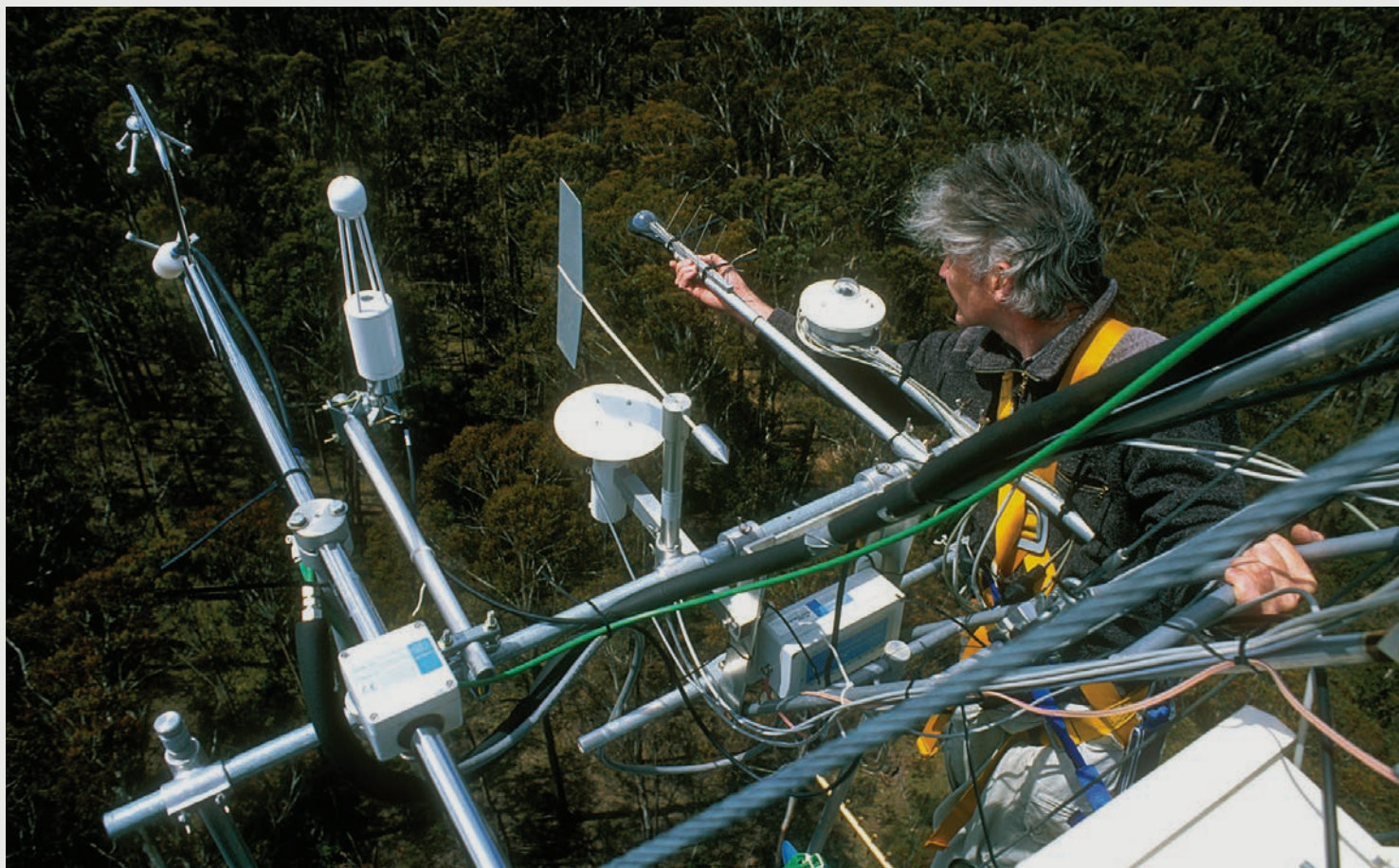
The Tumbarumba flux station is part of a network of towers around Australia that continuously measures exchanges of carbon dioxide, water vapour and energy between the ecosystem and the atmosphere.
