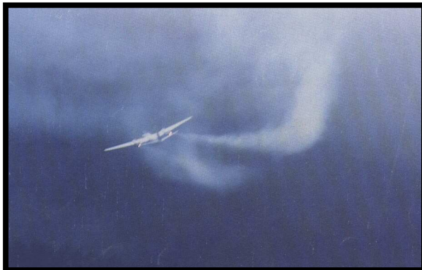
Figure 1. Aircraft dispensing hygroscopic seeding material, resulting in a visible trail of water droplets.
